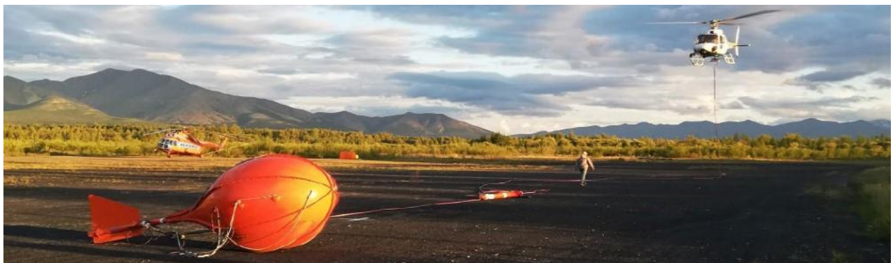
Figure 3: Heliborne Mobile MT Survey Showing Towed Bird (source: EGL archive)
